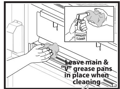
INTERIOR COMPARTMENT – Spray cloth with degreaser or approved oven cleaner, then wipe walls
